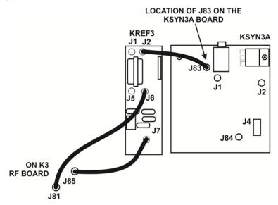
**Page A-5 (Parts List):** The "New KSYN3A Synthesizer" image above replaces the synthesizer shown. Change the part number of the synthesizer to E850638.
